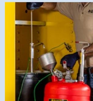
Use drum pumps to safely transfer hand sanitizer into intermediate containers. Includes pre-assembled bonding and grounding clamps to help control static discharge.
