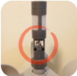
showed in the picture, the filter with white film can be easily pull up. The sensors it protects are marked in the red circle.
