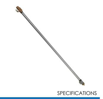
Model MK8A is a special freeze-protected valve that drains water from Model 8300FP combination shower/eyewash after closing to prevent freezing. 3/4" NPT inlet. Standard sizes are 60" and 78" (152.4 and 198.1 cm) for bury depths of 24" and 42" (61 and 106.7 cm) respectively. Servicing Instructions: For replacement of damaged parts, order the VRKMK8A repair kit which includes packing, stuffing box, stuffing box nut, spring and plunger assembly with four O-rings.
