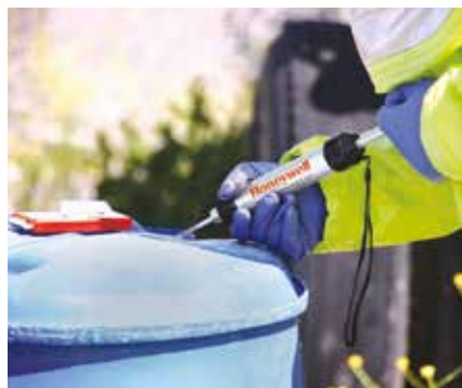
First responder uses Honeywell Colorimetric Tubes and Hand Pump to measure VOC levels inside a barrel.
