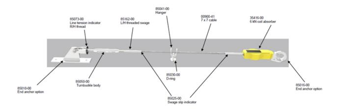
The user, wearing a full body harness and energy absorbing lanyard, is continuously attached to the system via a Latchways Transfastener, MSA's innovative device that can rotate through the intermediate cable supports. For systems with no entry terminal, a Removable Transfasterner can be used.
