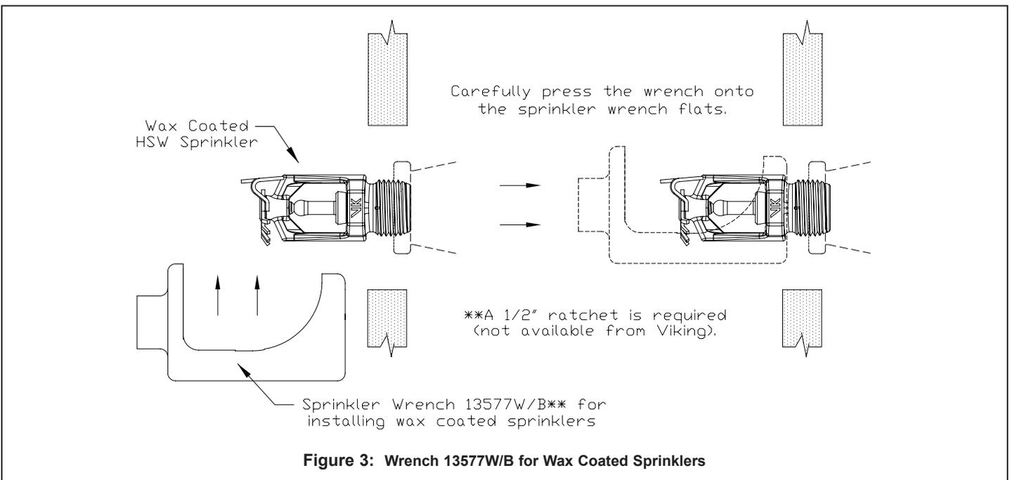
Figure 3: Wrench 13577W/B for Wax Coated Sprinklers
