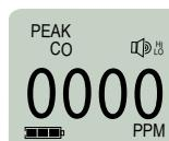
The T40 Rattler is equipped with audible, visual, and vibrating alarms to alert you when the ambient gas concentration exceeds one of the two alarm levels (low and high). For CO, the T40 Rattler is preset to alarm at 35 and 70 ppm. For H<sub>2</sub>S, the preset alarm levels are 10 and 20 ppm. To change these low and high settings, see 'Setting the Configuration' below.
