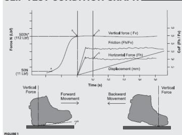
Based on bio-mechanical studies by SATRA Technology Centre, Timberland recommends selecting a shoe based on the contaminant and floor surface you will encounter that achieves at least a 0.3 Dynamic CoF using a Whole Shoe Test Method.
