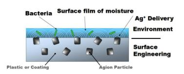
Zeolite particle delivers Ag\* over short range Does not require direct contact with treated surface When moisture dries, Ag\* is complexed in low-solubility compounds
