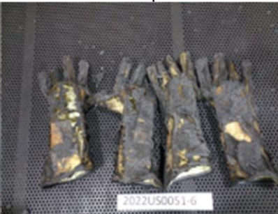
Ignition withstand verification – After exposure
