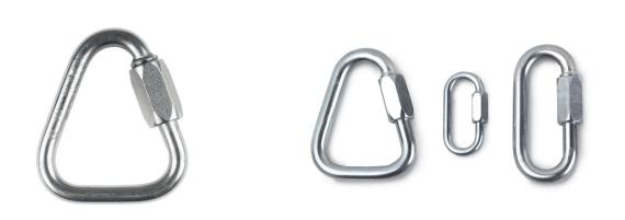
Quick Links, or also commonly known as screw links, are gaining popularity for use in situations for which carabiners are not recommended, such as when tri-axial loading cannot be avoided. The Delta shape can be used to rig anchors. The Delta can be used as a chest harness connector. While slower to open and close than a carabiner, they can be more secure when tightened down — and they cost less.
