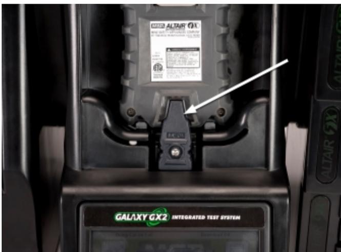
2. If using the charging option on the ALTAIR 4/4X instrument ensure the Test Stand charging connector at the bottom of the cradle makes contact with the instrument contact.
