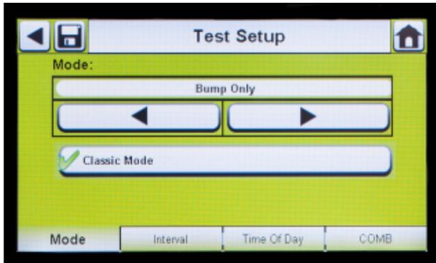
If the user disables the Classic Mode (✗) and datalog downloading is enabled, the Test Stand will determine if testing is due based on the last test date and the interval. If not, the Test Stand downloads the datalogs.
