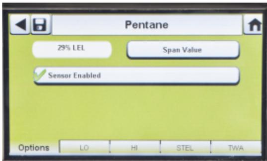
2. Select the **sensor** that you wish to configure on the Sensor Setup screen.
