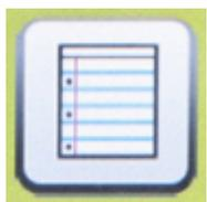
Provides the most recent calibration and/or bump record for each instrument in the Test Stand bank. **This button is only active on the Master Test Stand and only if an SD card is inserted.** All other Test Stands will report their data to the Master Test Stand for display. Each record uses 1 kB of memory. The number of records that can be stored depends on the SD card size.
