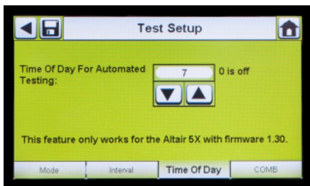
1. Select the up and down arrow keys to set the time of day on the 24 hour clock. Selecting 0 turns the feature off. Selecting 24 will initiate testing at midnight.
