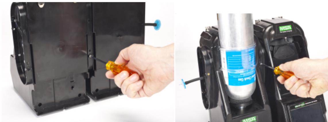
4. If connecting multiple Test Stands, remove the white gas plugs [→ [Figure 3](#)] from all units except the farthest right Test Stand. If using ammonia or chlorine test gas, read the restriction found under chapter [2.7 Special Conditions for Use with Reactive Gases](#) regarding the white plugs.
