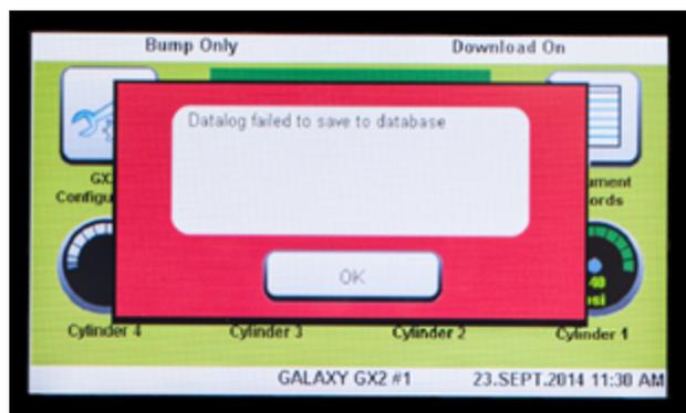
If the datalog does not save to the database, check your network connection to the GX2 Connect service.
