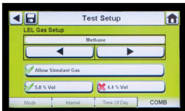
1. If the gas detector contains a combustible (COMB) sensor, select the %volume to 100%LEL conversion for each gas type. This conversion factor is determined by regional regulations.
