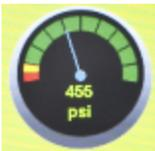
Display test gas cylinder pressure **from the electronic Cylinder Holder only**. Selecting a pressure gauge displays gas cylinder details.
