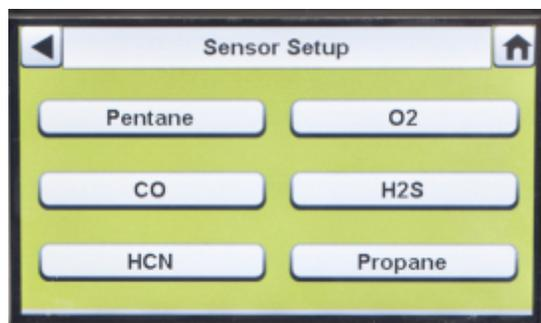
1. Select **Sensor Setup** from the Instrument Configuration screen [→ [Figure 16](#) ].
