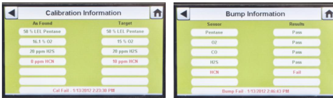
**i** If the instrument fails the bump test while the mode is set to **Bump/Cal on Fail** the Test Stand will automatically calibrate the instrument.
