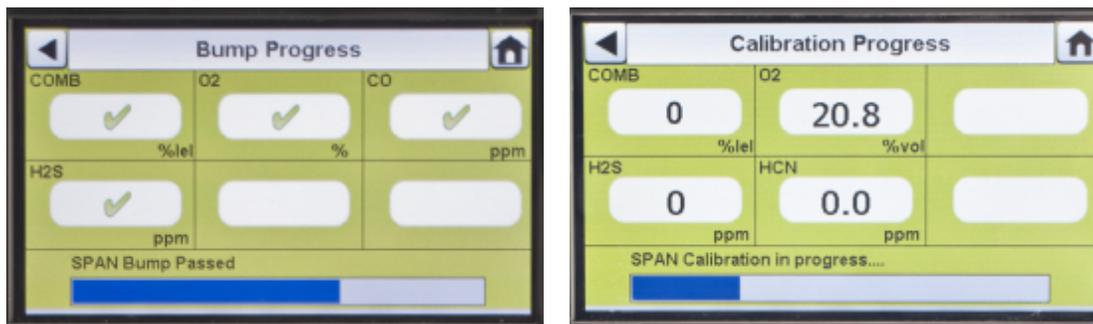
For the Bump Progress screen, an hourglass symbol will display in each sensor box until that sensor's bump is complete. A green checkmark (✓) or red X (✗) will display for each sensor when the Bump test is complete.
