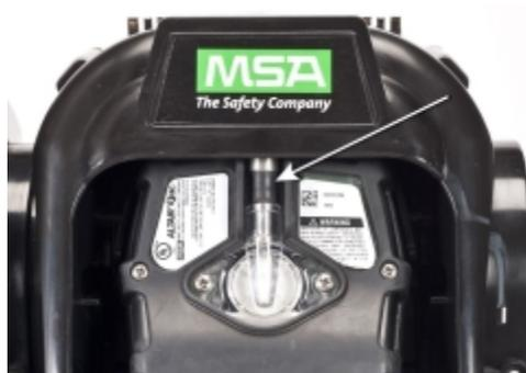
2. Pivot the instrument in the cradle upwards, into the gas inlet sleeve (see arrow). The instrument will lock into place, once properly positioned.
