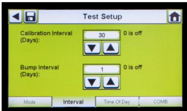
3. Select the up and down arrows to set the Calibration Interval from 0 to 180 days.
